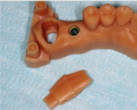
Superior and inferior quarter printed with DWS PRECISA RD097, specific for highly accurate models and in 3D printer DWS DW020D.
