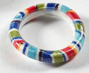
A nanoceramic material to create objects recalling the same properties of artisan ceramics: a blank canvas where unleashing your chromatic creativity. The material resists at 180° C, and, after the coating in enamel, in various customized colors, must be placed in an oven to obtain a result identical to porcelain.
