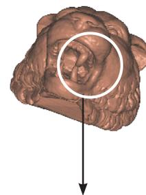
Recovers fine details from noisy or sparse scan data and intelligently detects, and automatically fills the holes.
