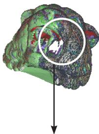
It is difficult to obtain scan data from deep and narrow parts of an object.
