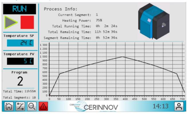
The console allows you to set the furnace's heating programs (thermal cycle) and to view the temperature monitoring and the electrical power consumed in real time.
