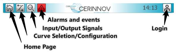
This section is always visible to the user. It allows you to select either the page to be viewed, or the heating curves, or to access and modify the parameters of the curves, or to access user accounts or to display events and alarms.
