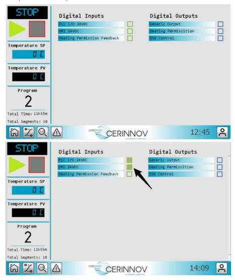
This page is intended for monitoring the system by allowing you to view the signals that the PLC receives and sends. It can be used to identify the absence of a signal such as:
