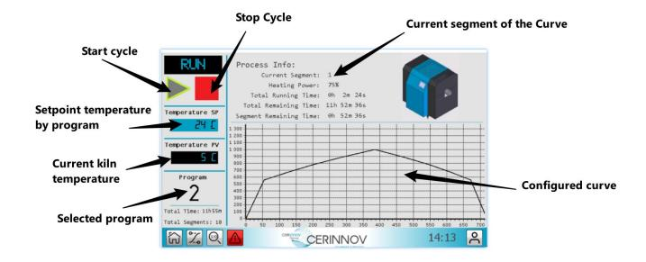
On the main page, you can start the cooking cycle, view the time left before the cycle ends as well as the current temperature and set temperature.
