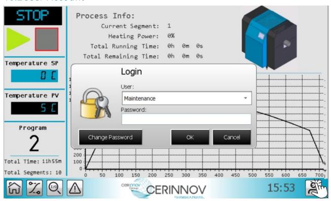
Setting up thermal cycles requires logging in with the "Maintenance" account. The default password is 0.
